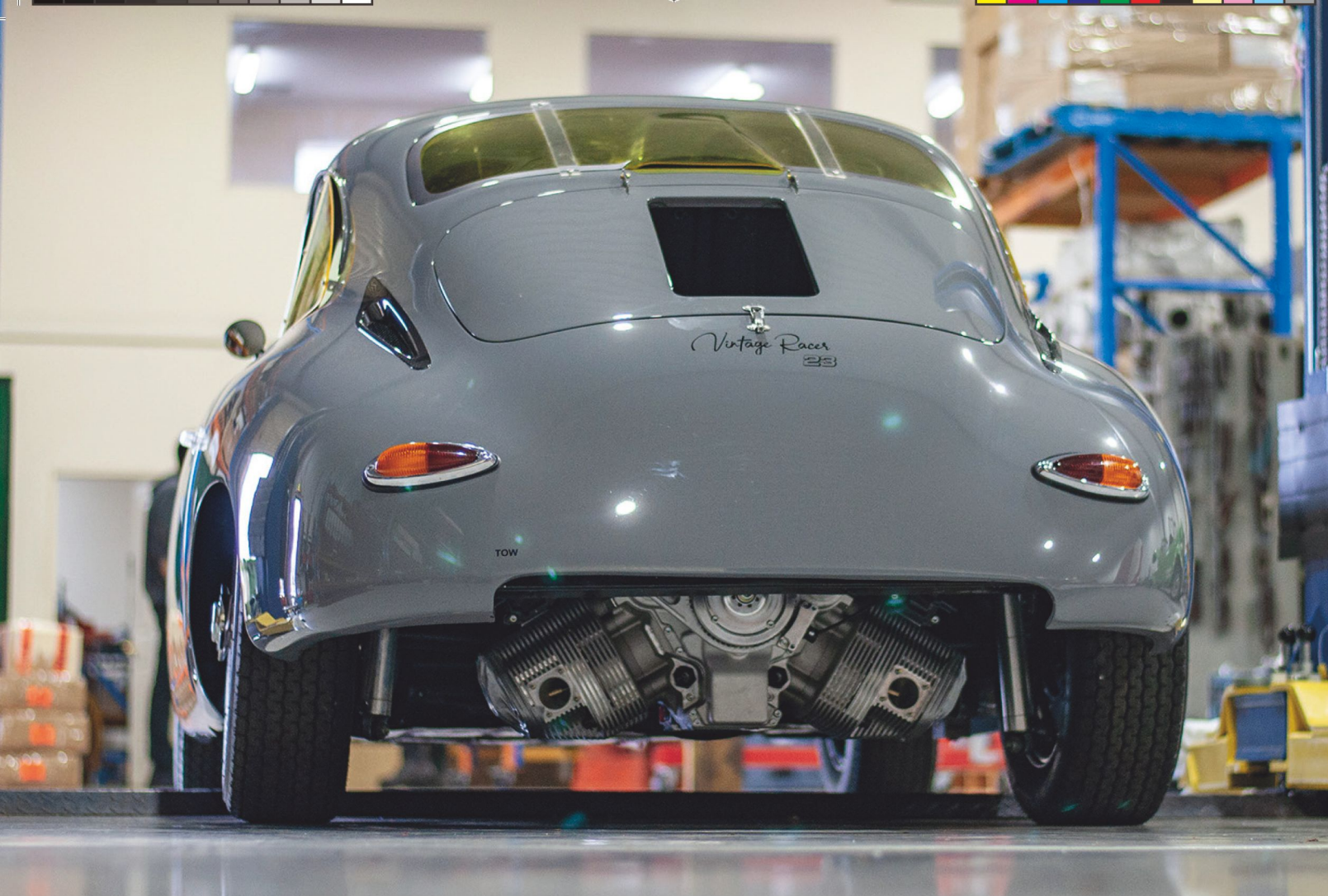
Above Radial Motion three-cylinder engine is perfectly suited to older classics with limited engine bay space
